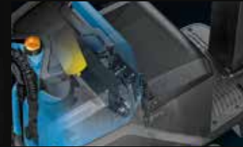
On-board Battery Charger
